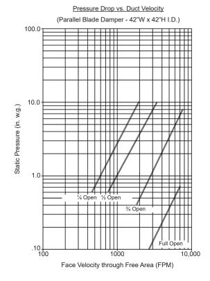
Industrial Damper • 10" Deep • 8" Insulated Airfoil Blades • Galvanized Steel Channel Frame • 200°F Max Temperature
